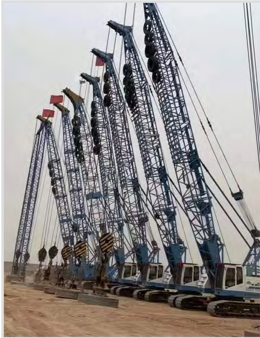
宇通液压履带式强夯机YTQH400A
